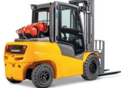
Diesel/LPG forklift truck DFG/TFG 540-S50 hydrodynamic max. lift height: 7,500 mm max. capacity: 5,000 kg
