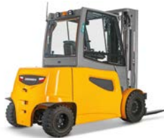
Electric 4-wheel counterbalance truck EFG 535k-S50s max. lift height: 7,500 mm max. capacity: 5,000 kg
