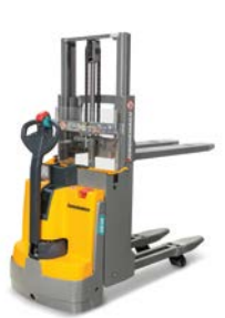
Electric pedestrian stacker for double deck loading EJD 118/220 max. lift height: 2,560 mm max. capacity: 2,000 kg
