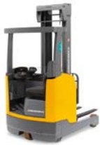
Reach truck ETM/ETV 214/216 max. lift height: 10,700 mm max. capacity: 1,600 kg
