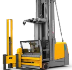
Order picker/tri-lateral stacker EKX 410-412* max. lift height: 11,500 mm max. capacity: 1,200 kg
