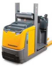
Vertical order picker EKS 110 max. picking height: 4,600 mm max. capacity: 1,000 kg
