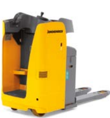
Electric stand-in/sit-on pallet truck ESE 120 max. capacity: 2,000 kg
