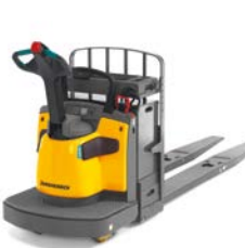
Low level order picker ECR 327/336 max. capacity: 3,600 kg
