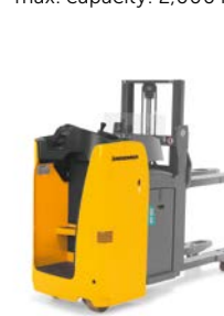
Electric stand-on and sideways seated stacker for double-deck loading ESD 120/220 max. lift height: 2,560 mm max. capacity: 2,000 kg
